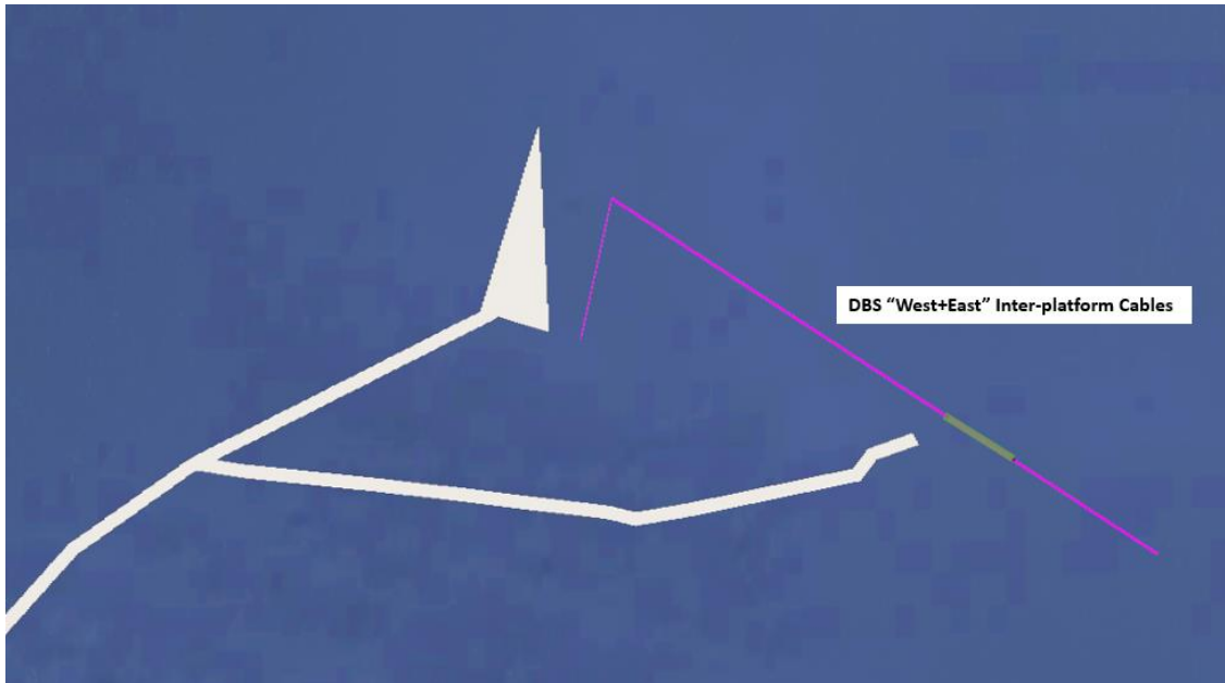
Figure 8-3-33 Inter-Platform Cable Routes for DBS “West and East” Routes (green lines indicate areas requiring seabed levelling) 9
