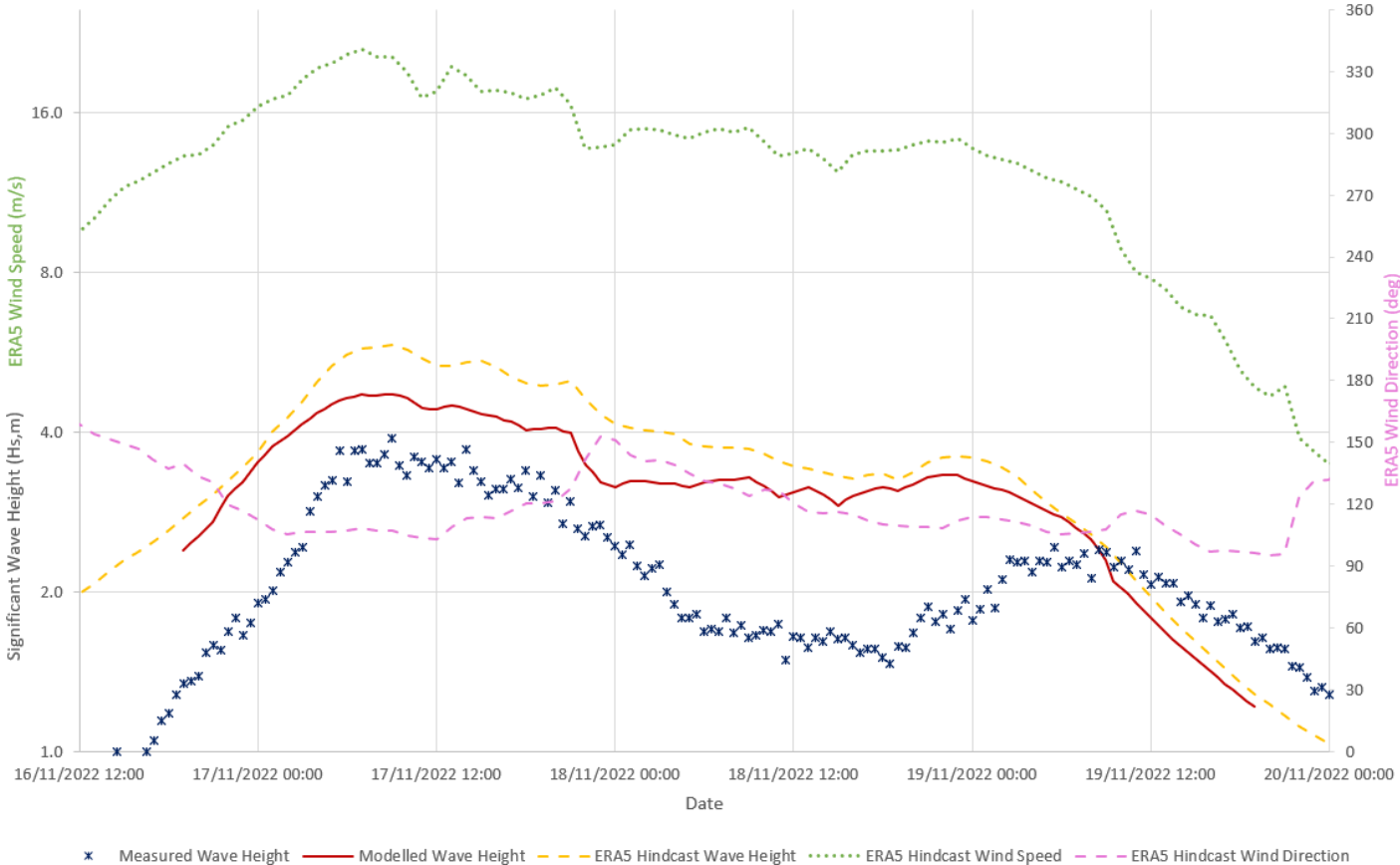
Figure 8-3-8: Comparison of Measured and Modelled Wave Height at Hornsea Wave Buoy for Waves Approaching from the East.
